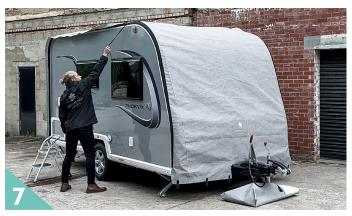
Once the top panel is in place starting at the front of the caravan pull the zip along the roof line. This is again easier with ladders or a step and we have added an additional strap to the zip pull to support moving it along the caravan.
