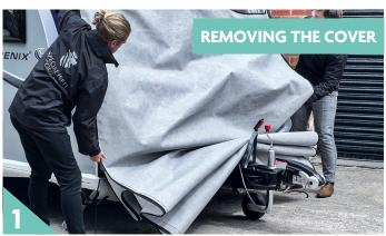
To remove the cover undo the leg steady straps from all four corners and unzip the cover on both sides.
