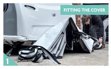
Remove the cover and straps from the bag placing the open cover over the A-frame.
