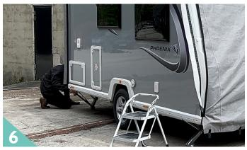
When you reach the back of the caravan loosely fasten the leg steady straps around the legs to prevent the cover from moving whilst you secure the zips.
