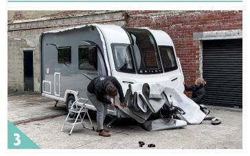
Feed the awning tape into each of the awning channels on both sides of the caravan leaving the folded section of the cover on the a-frame. Feed the awning tape all the way to the back of the caravan.
