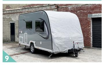
Ensure that the A-frame strap is secured and any excess webbing is removed. The rear leg steadies can be adjusted at this point if not done previously. Check the zip covers are over the ends of the zips and you are happy the cover is secured.
