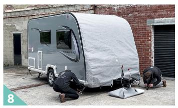
When both sides are fully zipped up the leg steady straps can then be added. The supplied straps should be clipped into the front middle buckle, threaded through any section of the leg then clipped in the buckle closest to the awning rail.
