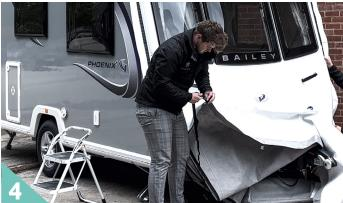
Once the awning tape is in on both sides secure the rear leg steady straps to the rear clips which should currently be at the front of the caravan and are located on the rear of the cover.
