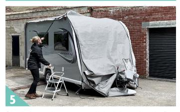
Once the leg steady straps are attached walk down either side of the caravan lifting the top panel as you go down. Please be aware of aerials and other items that are on your roof, as the cover will need to be lifted over these.
