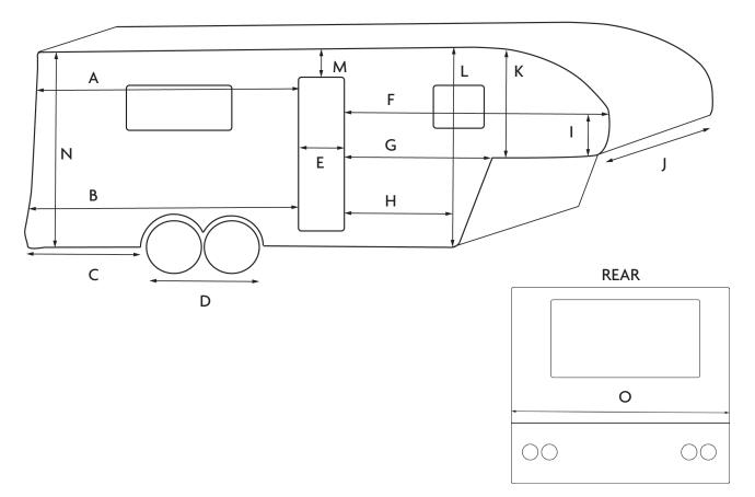
If you have roof elements to note, take a single length measurement from the back of the Caravan along the Gutter Line.
