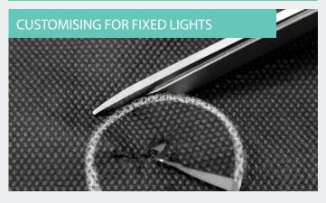
Once you have marked the new light on the TOW PRO LITE cut around the outside of the marking. This may need to be trimmed and refined to secure the rings in place and fit accurately.
