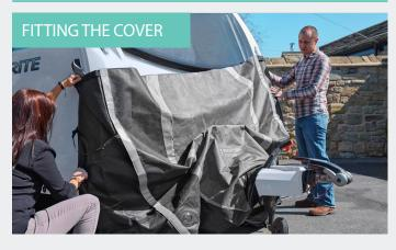
Insert the TOW PRO LITE into the awning channels on either side of the caravan - the same way you would do an awning. Slide the cover either up or down the channels, depending on your opening's location, until it sits neatly on the A-frame section.
