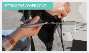
Simply cut along the tube edge but not the tape section the height of the awning stopper. Once the tube has been removed this will allow the excess awning tape to lay flat over the stopper.
